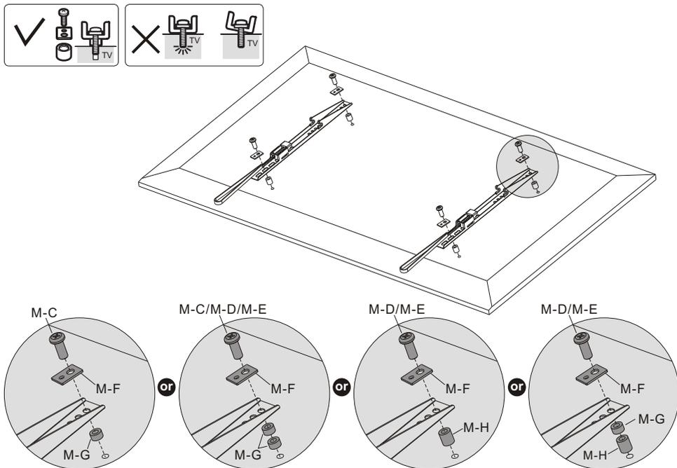
**Note:** Choose the appropriate screws, washers and spacers (if necessary) according to the type of screen.
